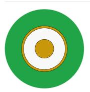
Cable Application: CATV cables are used in trunk lines of CATV and broadband networks between head-end and subscriber termination point. They are suitable for direct buried and duct laying.
