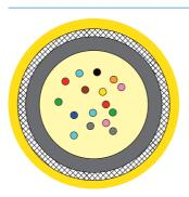
Cable Application: This uni tube dielectric optical cable is designed for outdoor installation in ducts and micro ducts by blowing techniques.
