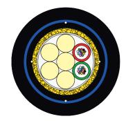
Cable Application: This dielectric optical cable is designed for duct or direct buried installation technique.
