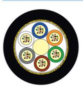
Cable Application: This mini Flextube dielectric optical cable is designed for outdoor installation in duct by pulling, jetting or floating technics. Mainly used for distribution and access network. The FlexTube® design provides easier storage & faster installation. Finger access to the fibres: no specific tools to open the FlexTube®.
