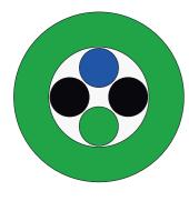
**Cable Application:** This Pico-TX optical cable is designed for blowing in 2.5 to 3.5 mm inner diameter microducts and for preinstallation in ducts, used in OSP networks access part of the network.
