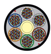
**Cable Application:** MassLink™ with FlexRibbon™ Technology provides a compact outside plant cable design that contains 864 bend insensitive fibers for access or data center applications. By using FlexRibbon technology, ribbons are rolled up and packed together in small diameter 144 fiber sub units. While FlexRibbon™ provides high packing density, these 250 µm fiber ribbons still provide the advantages of mass fusion splicing.
