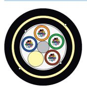
**Cable Application:** The cables are suitable for aerial installation, with 250 meters span and 2.0% installation sag. The cables withstand the additional loads generated by wind and ice in the following environmental conditions: temperature -10°C, wind speed 19m/s, ice radial thickness 18 mm. The use of Spiral Preformed fittings is recommended, in order to achieve the mentioned performance.
