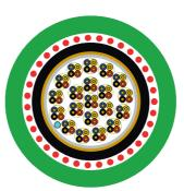
**Cable Application:** Polyethylene insulated cables for both instrumentation and telecommunication applications with overall screens and optionally incorporating various armouring and sheathing constructions. The screen provides protection from electromagnetic radiation coming from nearby electrical equipment, power lines, lightning strikes, transformers etcetera.
