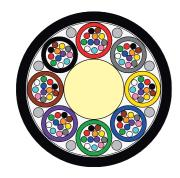
**Cable Application:** This loose tube dielectric optical cable is designed for outdoor installation in ducts and microducts by blowing or pulling techniques.
