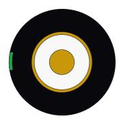
**Cable Application:** CATV cables are used in trunk lines of CATV and broadband networks between head-end and subscriber termination point. The HF-version is intended to be used in-house in cases where long reach and an advanced performance of reaction to fire is needed.
