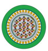
**Cable Application:** This cable is designed for outdoor installation allong railway lines. The design with copper wires improves the EMC characteristics. This design also replaces the PIWY cable construction and is suitable for connections with the existing networks.
