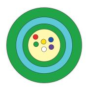
**Cable Application:** This unitube dielectric optical cable is designed for direct buried installation, surrounded by sand. As a result of temperature changing, especially when used above ground, fibers and gel may be pushed out of the cable. Connectivity materials should be able to accommodate that or Prysmian may offer other cable designs for such above ground applications.
