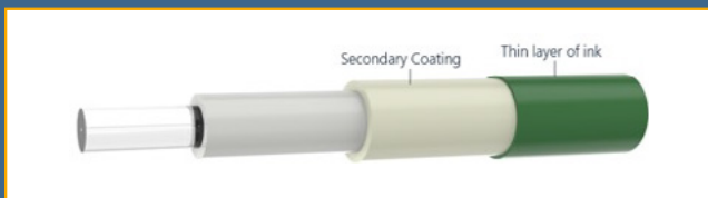
Diagram 2: Example of a UV inked optical fiber.
