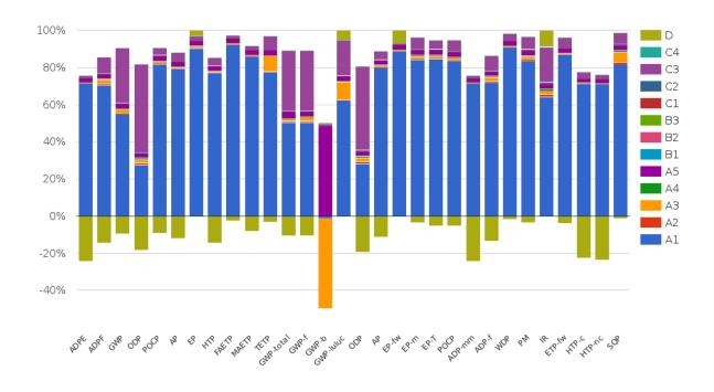
The most significant contribution is from the raw materials in A1. This is offset by the contribution (benefit) in module D. The metal (copper) is very well recyclable and because of its value it is always recovered. The plastics in the product are recovered from production waste, but not End-of-life. Because there is no return program for the product end-of-life the default EOL scenario's are used and these still consider mostly incineration as EOL process.
