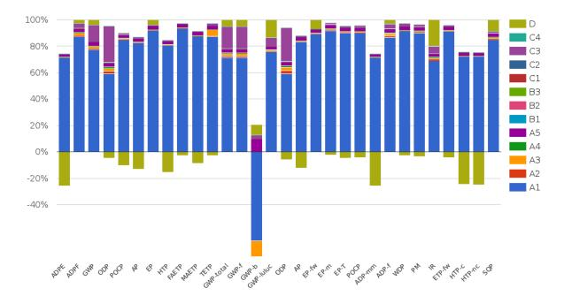
The most significant contribution is from the raw materials in A1. This is offset by the contribution (benefit) in module D. The metal (copper) is very well recyclable and because of its value it is always recovered. The plastics in the product are recovered from production waste, but not End-of-life. Because there is no return program for the product end-of-life the default EOL scenario's are used and these still consider mostly incineration as EOL process.
