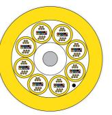
**Cable Application:** The intended application for this cable is as trunk net cable inside data centres and central offices. Fits 12 way multifibre connectors according to IEC 61754-7-1 such as the MPO® and MTP<sup>®</sup> connectors without the need for a fan-out gland.
