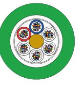
**Cable Application:** This dielectric optical cable is designed for duct installation technique.
