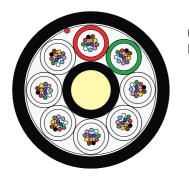
Cable Application: This dielectric optical cable is designed for blowing installation technique.
