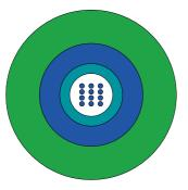
Cable Application: This cable can be used for LAN and WAN backbones, telecom access lines, fibre to business and fibre to the building drop connections as well as fibre to the home drop and access connections. With its FireRes<sup>®</sup> LSHF-FR sheathing this cable is ideal for indoor and limited outdoor installations. This cable features a high tensile strength and a degree of rodent protection, effective in many cases. It is equally suited for installation in ducts and on trays.
