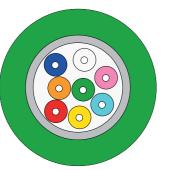
**Cable Application:** This distribution or mini breakout cable with FireRes<sup>®</sup> sheathcan be used for many indoor applications. Typical cable applications include: LAN and WAN backbones, central office interconnections, backbones in data centres, and many other. This cablefeatures high flame retardance with CPR Cca approval.
