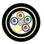
**Cable Application:** The cables are suitable for aerial installation, with 250 meters span and 2.0% installation sag. The cables withstand the additional loads generated by wind and ice in the following environmental conditions: temperature -10°C, wind speed 19m/s, ice radial thickness 18 mm. The use of Spiral Preformed fittings is recommended, in order to achieve the mentioned performance.
