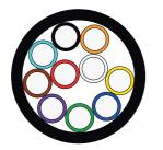
**Cable Application:** Highly reliable, robust protective flexible ducts with pre-installed high pressure resistant microducts with superior blowing capabilities. The flexible ducts are made of a special grade polyamide, offering excellent protection: • mechanical protection, • flame retardancy • chemical resistance. The application area is indoor, typically for high-rise buildings.
