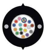
Cable Application: Indoor installation on cable tray, in corridors, shafts or aerial installation with 15m span. Easy selection and removal of a tube for tapping and connection at the floor. The fully dry flexible micro-modules provide easier storage & faster installation and access to the fibres with specific tools and without further cleaning. The minimum strip-ability of the modules is 30 cm.
