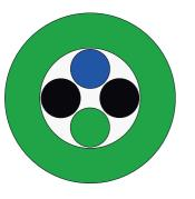
Cable Application: This Pico-TX optical cable is designed for blowing in 2.5 to 3.5 mm inner diameter microducts and for preinstallation in ducts, used in OSP networks access part of the network.
